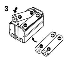
**Note:** When the set is not to be used for a long period of time or is to be operated extensively on other power sources, remove the batteries to avoid set damage caused by battery leakage and corrosion.
